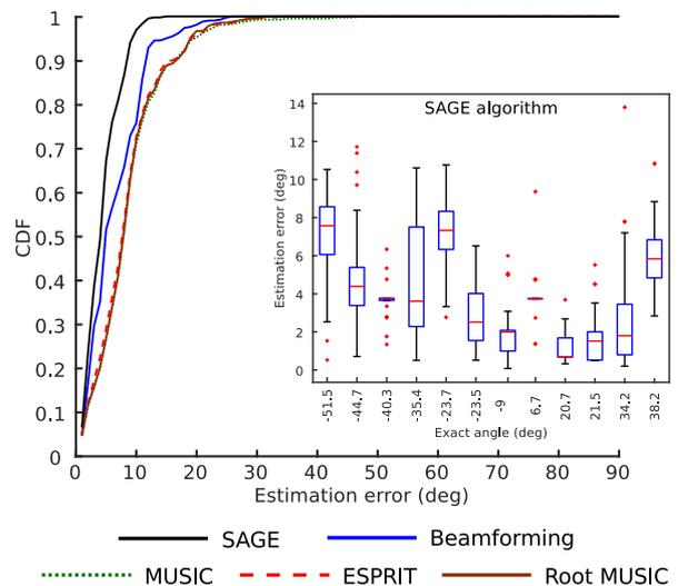
**Fig. 2: The CDF and the boxplot (inner figures) graphs for the AoA estimation error of all the received signals from the LoS and the NLoS locations, respectively. The CDF figures show the AoA estimation error as estimated from all the deployed AoA estimation algorithms. The boxplot figures, on the other hand, provide the AoA estimation error from the SAGE algorithm only. Every boxplot represents the estimation error from a specific location (i.e. 26 boxplot graphs in total).**
