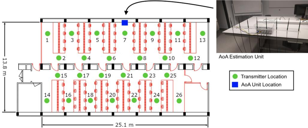
**Fig. 1: The experimental setup. It constitutes two parallel computer classrooms of dimensions  $25.1\text{m} \times 6.9\text{m}$  each. 780 DASH7 signals were transmitted from 26 different locations in both rooms (30 signals per location). The two parallel classrooms were full with computer screens, therefore, this environment can be considered a rich multipath environment. Furthermore, the wall (that is separating the two classrooms) provides a physical barrier between the two rooms.**
